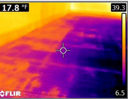
Infrared image of mositure-damaged
